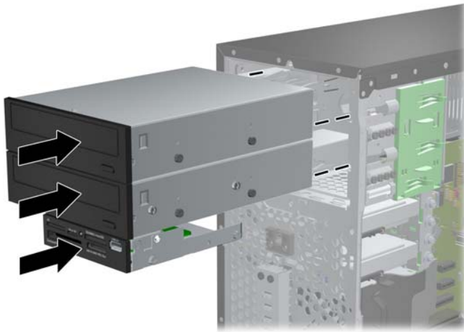
Figure 3-22 Sliding the Drives into the Drive Cage
